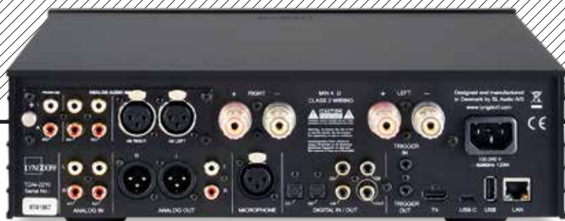
ABOVE: Seen with the optional MM phono/balanced line 'Analogue' module, the TDAI-2210 includes two optical, three coax, USB-C, USB-A (storage) and wired/wireless Ethernet inputs alongside HDMI eARC. Single speaker outputs are joined by balanced preamp outs and a 96kHz digital coax out. An XLR mic input serves RoomPerfect
