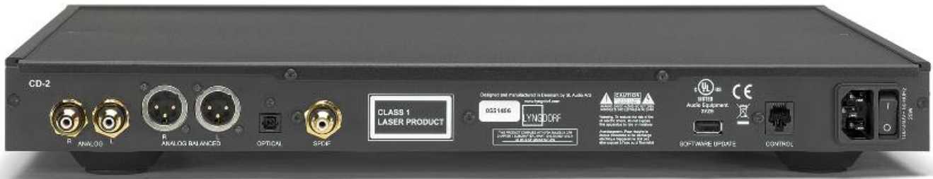
The rear panel with the analogue outputs on the left, the optical and coaxial digital outputs as well as the hard power switch and the mains socket on the right. The CD-2 comes with a decent mains cable
